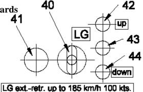
40) Toggle switch for extension and retraction of the electrically operated main landing gear
