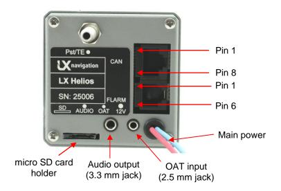
Pin out on all connectors: Pin 1 to pin 6 or 8 (on picture from top to bottom).
