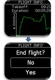
During flight, statistic of the flight is shown on statistic page. Take-off and duration time are displayed on top with baro altitude graph for last hour at the bottom.
