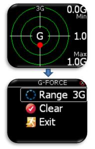
During the flight red dot of G-force page is showing current detected Gforce. On right top and bottom corners, minimal and maximal detected Gforce during the flight are displayed. This values can be cleared anytime during the flight in G-FORCE menu. In the middle, current G-force value is displayed. Range setting is presented with small text on top of G-force scale (example is showing 3G range). This range can also be set in G-FORCE menu.
