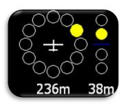
When flarm warning is detected, Eos will show Flarm warning page with direction, above/bellow indicator and numerical information for distance and relative altitude.
