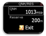
Pilot should set actual QNH and elevation of the airport where he will take-, off on initial setup screen. After change of QNH during flight, pilot can change altitude information to which final glide will calculate. If QNH is changed on the ground, altitude will not be corrected and will still be the same as set on initial setup.
