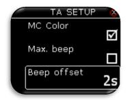
Thermal assistant page can assist pilot when thermaling to get better sense how thermal looks like. Thermal is presented with use of different coloured dots.
