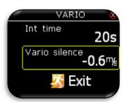
Vario silence will define the value of vario bellow which vario sound is muted. In this example, vario less then -0.6m/s will not generate vario beep. This option can be set to OFF.
