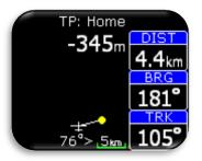
On the top of this page pilot can find name of navigated TP. Under the name, final glide (FG) information to the selected point is visible. Final glide uses reserve altitude in end result. Navbox-es shows track (TRK), bearing (BRG) and distance (DIST) to the selected point.
