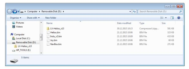
Insert SD card to the SD card holder of LX Helios (in the back side). Press and hold power on button until you will see Helios start up screen with new version details. After that you can release power on button. This procedure usually takes about 1min. If you release power on button too soon, update will not be finished correctly and you will have to press on button again and hold it down until start up screen will be visible. After that restart the unit and power it on again.
