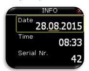
Pilot can set current date and time under info page. If GPS source is connected, date and time will automatically be set. Date and time should be set to UTC.
